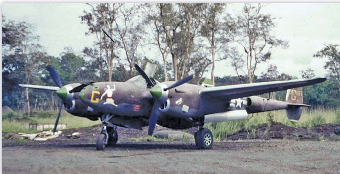
P-38J 42-67587 Princess Pat II seen at Nadzab. This aircraft replaced Princess Pat which is depicted in Profile 61. Note that the letter G has been painted over the tail serial, rather than removing it first.
