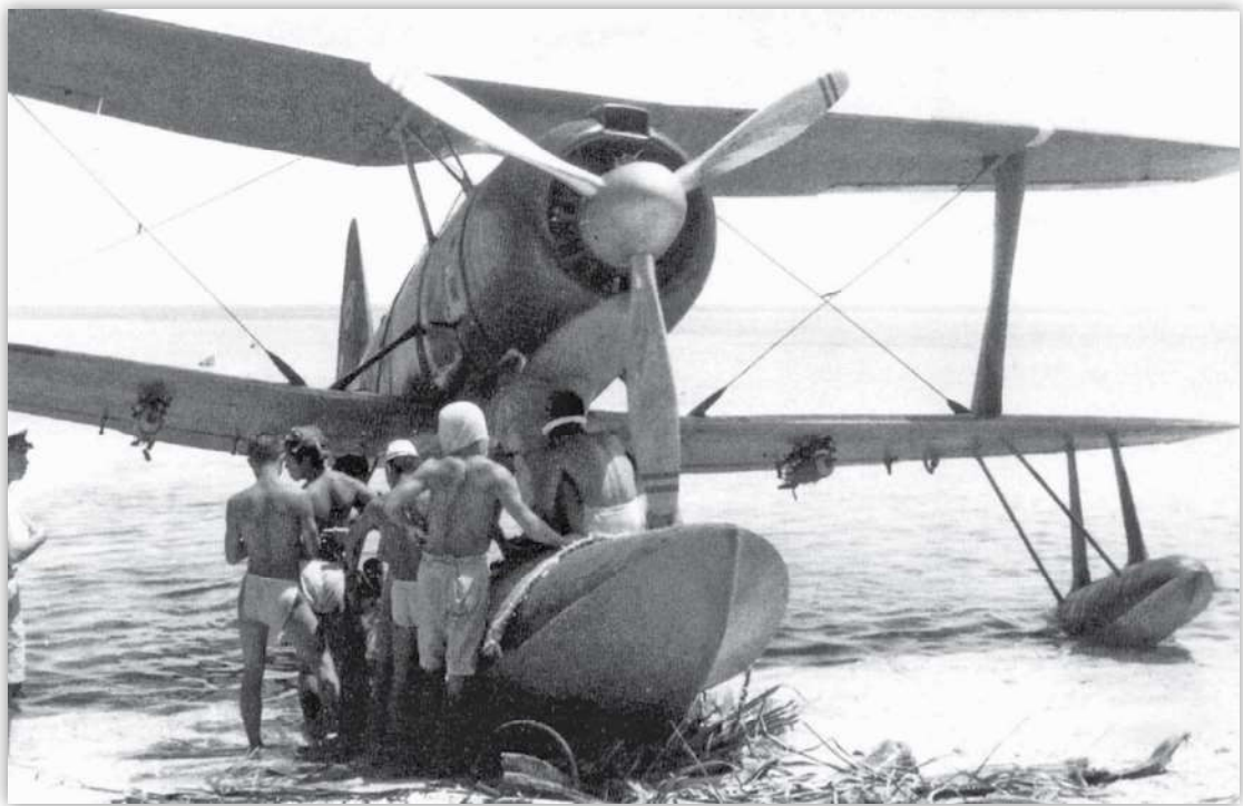
At Poporang an officer gives orders to sailors who are retrieving Pete L-2-8 after an operational flight. Note the two small 30-kilogram bombs slung under the lower wings.
