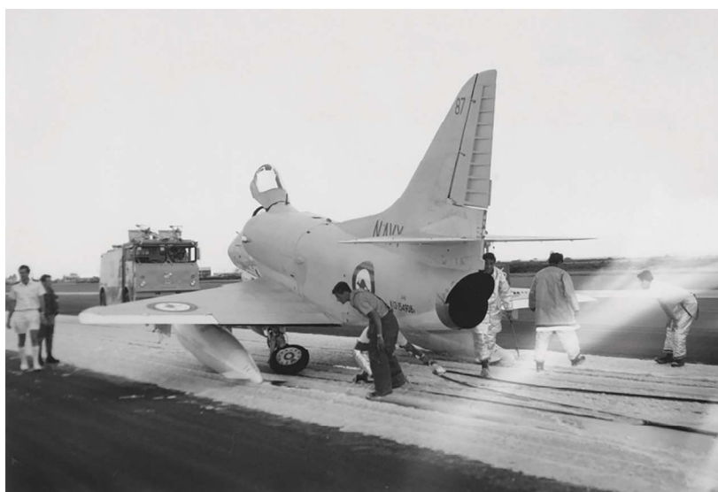
John Hamilton's aircraft after a short-field arrest on its tanks at NAS Barbers Point, Hawaii, on 27 October 1971. The officer in short summer whites is the AEO. (FAAAoA)
