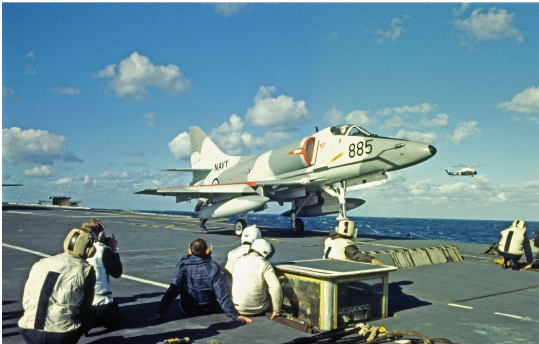
Skyhawk 885 taxiing forward in the initial stage of being loaded on the catapult. Note the plane guard Wessex in the background, positioned approximately 400 metres off the port quarter as described by Dick Chartier. Note also the camouflage. By 1980 the Melbourne embarked a mix of camouflaged and non-camouflaged Skyhawks. The scheme had been first applied on a VC724 A-4 at Nowra in 1977 using washable paint. After formal approval, the scheme was applied by Qantas as airframes were overhauled. (Seapower Centre)
