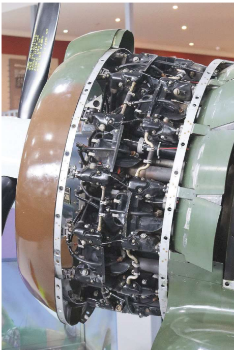
The Twin Wasp engine in A46-122, showing the two rows of cylinders. (Author)
