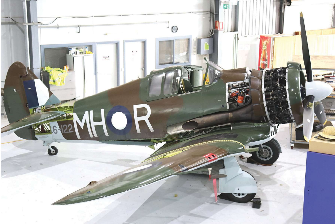
A46-122 being serviced at the Temora Aviation Museum. Visible are the Twin Wasp Engine, open cooling gills immediately behind the engine and straight-through engine exhaust. Part of the fuselage tubular framework at the tail can also be seen as well as the location of the join between the wing centre section and the outer wing section. (Author)
