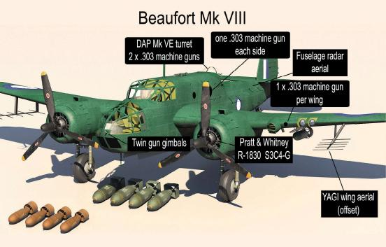
A comparison of the armaments of the Beaufort Mk V and Mk VIII. The Mk V was the initial production version, but the Mk VIII was the main production version and had a heavier machine gun armament as well as radar.
