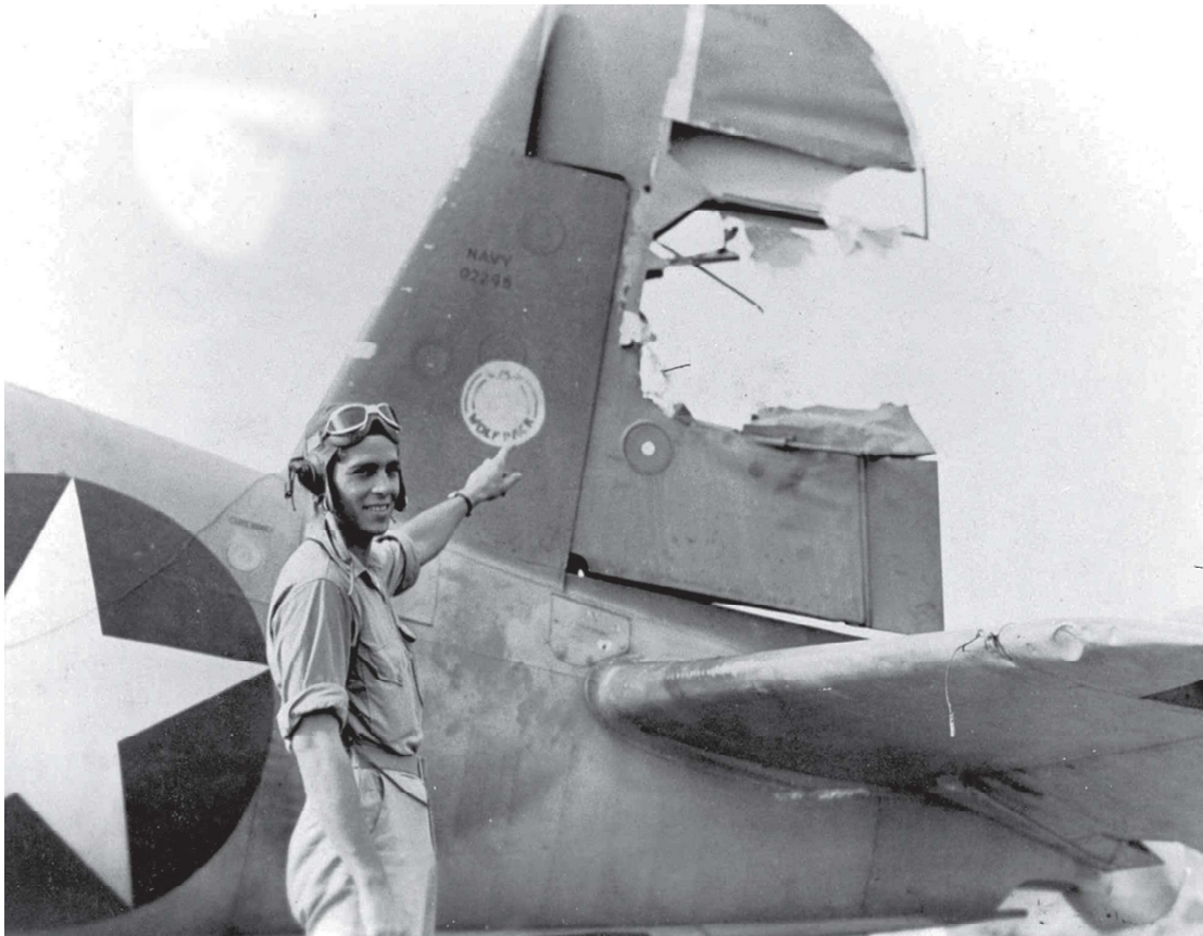
VMF-112 pilot Lieutenant James Johnson points to the shot out rudder on his F4U incurred during the 7 June 1943 combat with Zeros over the Russell Islands.
