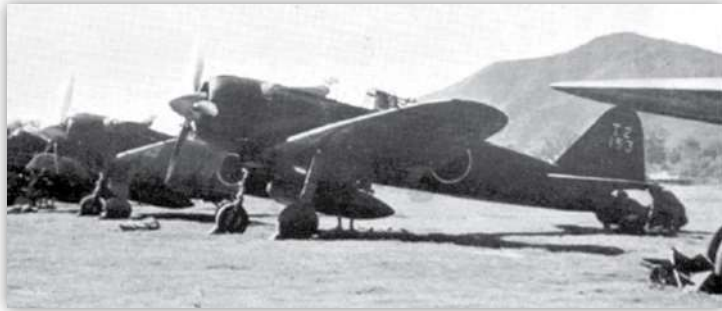
Zero T2 153 parked at Lakunai. This airframe and the one behind are both Model 22s.
