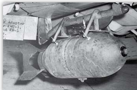
The crude but effective bomb rack built specifically by Brewster for the Corsair.
