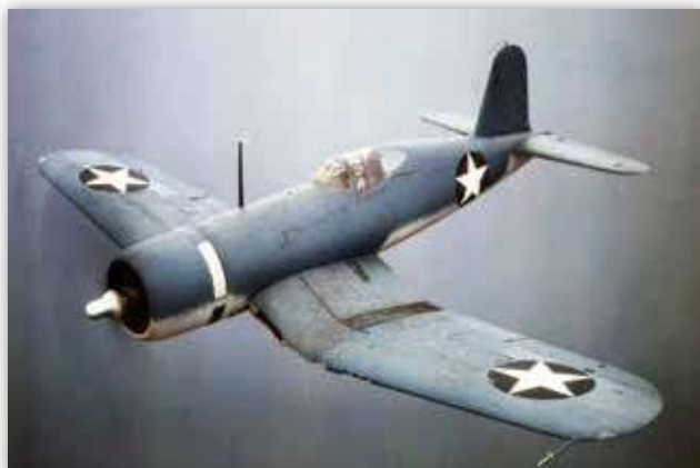
The first F4U-1 Corsair in flight over the US mainland in 1942, showing the two-tone blue-grey and light grey paint scheme. These were known as "birdcage" Corsairs due to the appearance of the canopy.
