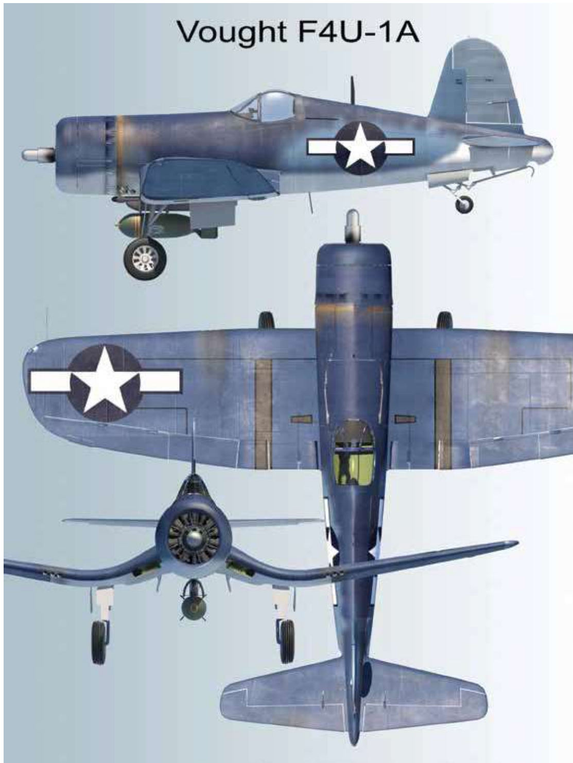
The Vought F4U-1A Corsair with its “bubbletop” canopy and three-tone colour scheme.
