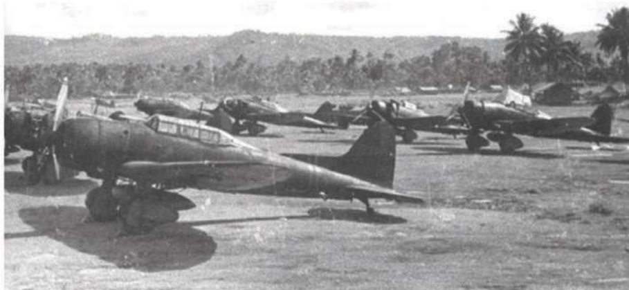
Junyo Vals at Vunakanau just prior to the Strike Y2 mission. Note the fuselage-slung fuel tanks, which meant only 60-kilogram bombs could be carried under the wings.
