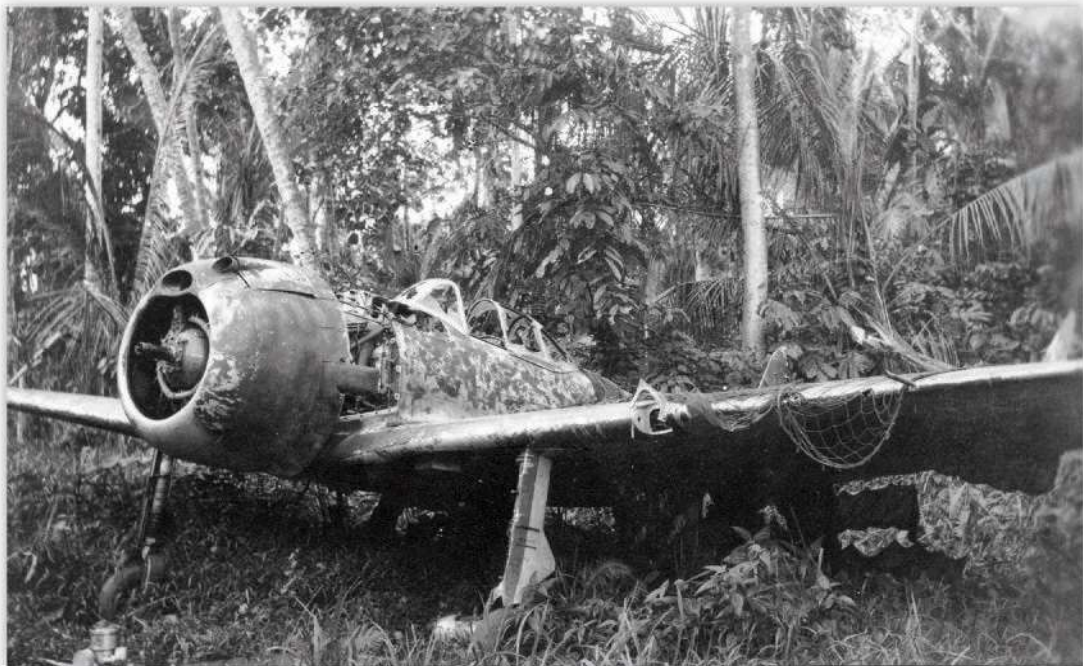
Ki-43-II MN 3958 seen abandoned at Dagua. It had a replacement cowl, as seen by the different camouflage marking. Note the camouflage netting draped over the port wing.
